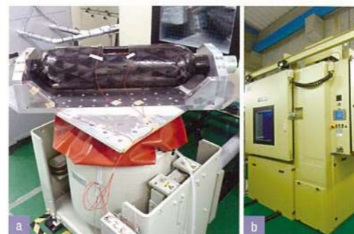
a/ Vibration test equipment b/ Environment and vibration test system
