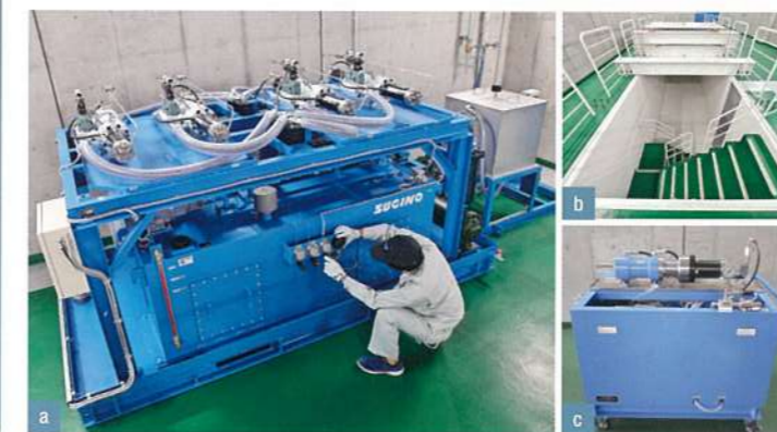
a/ Burst test system b/ Testing pit c/ Mobile pressure booster
