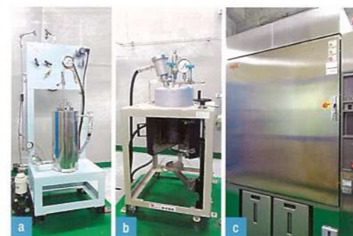
a/ High-pressure autoclave b/ High-temperature autoclave c/ Environmental test equipment
